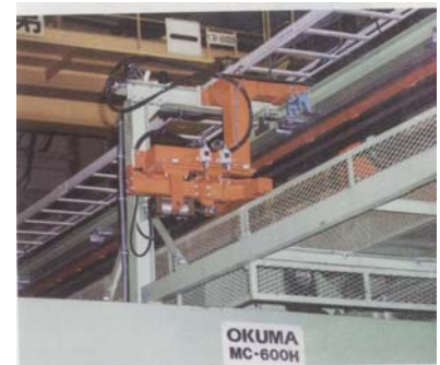
Photo 3: If a tool breaks in the FMS or is worn, the "Toolboy" changes it in the manufacturing system fully automatically.
