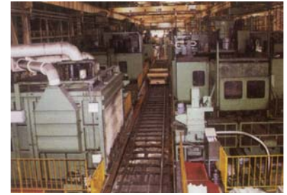
Photo 6: FMS from Double Column Machining Centers for the 5 page handling
