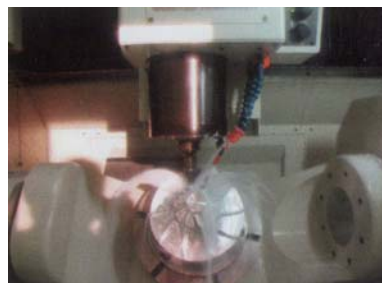
Photo 11: Handling impeller from Al on the 5-axes universal machining center MU-400 VA
