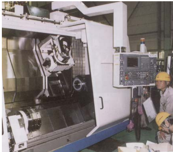
Photo 1: Here the turning and milling center MacTurn 250, is in the final assembly of the Okuma factory Oguchi, processes complex workpieces up to 1,000 mm lengthens and 250 mm in diameter in only one voltage fixed and ready to be installed. It summarizes turning, milling and machining and shortens the turn-around time also more compartment radically complex.
