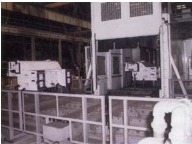
Photo 5: ... or with enormous pallet changer automatically operated
