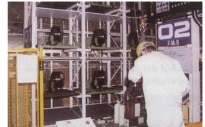
Photo 7: For the automatic production of machine tool turret is in Kani Machining Center and Lathe with a NC-loader connected to FMS
