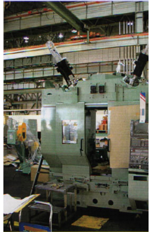
5 Parallel kinematics Cosmo Center under construction: from the few manufacturers of these machine conceptions, Okuma is the only one to already serve several users in the automobile environment
